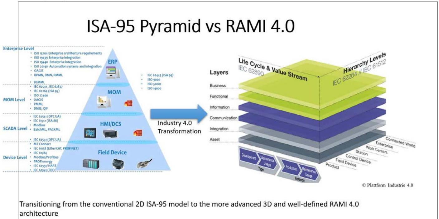
Figure 7: Lights-Out Manufacturing Levers - Process (ISA 95 vs RAMI 4.0 Architecture)
